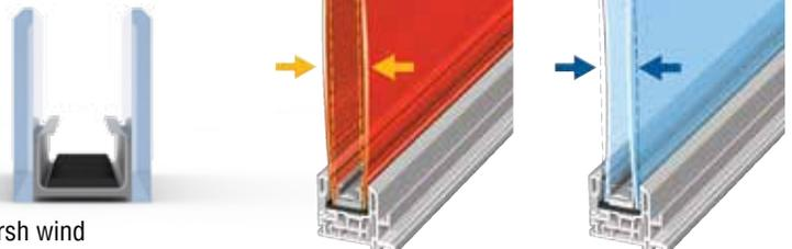
With conventional aluminum spacers, the sealant flexes, which can lead to sealant failure and loss of insulation performance. With the ClimaTech ThermD Spacer, IG units (insulated glass) flex instead of the sealant, thus resisting spacer movement and sealant failure.
